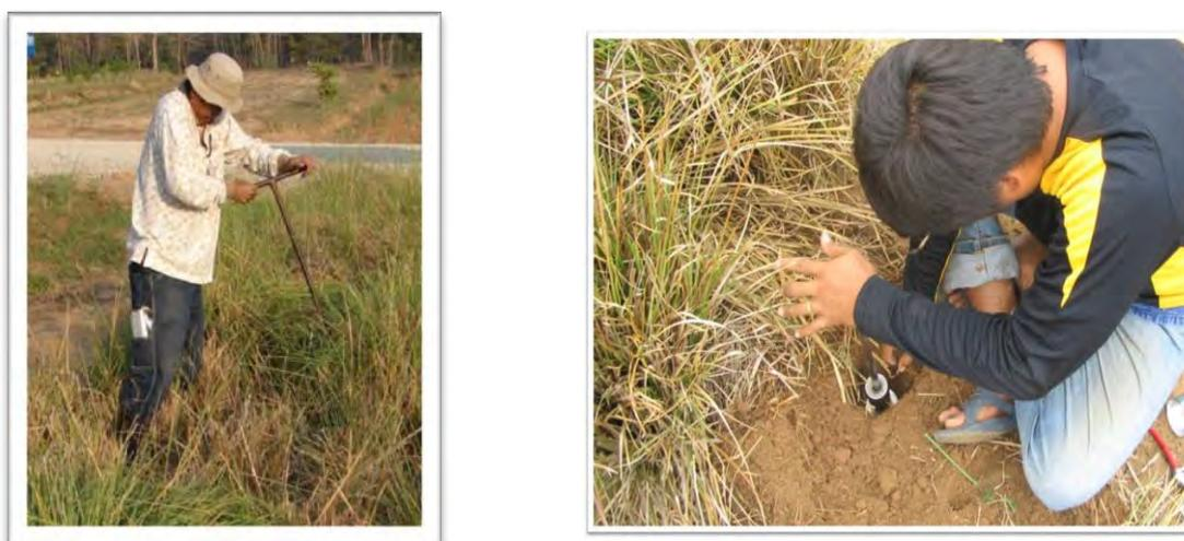
**Figure 3** Soil sampling and collecting of disturbed (left) and undisturbed soil (right)
