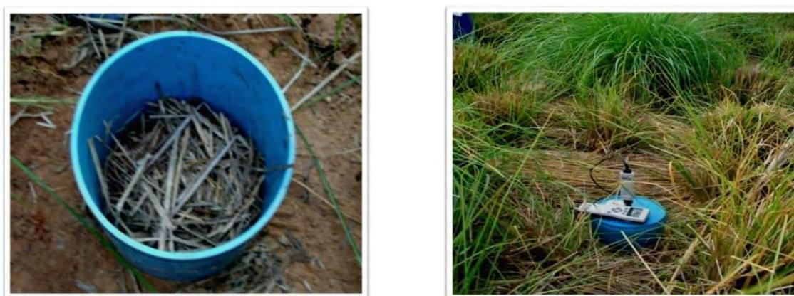
**Figure 4** Gas chamber (left) and measurement of CO<sub>2</sub> emission rate by Hand-Held CO<sub>2</sub> Meter (right)
